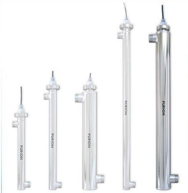
UV Plant PURION 2501 is equipped with a polished stainless steel reactor. PURION 2501 can be used to disinfect pool water up to a Volume of 50.000 l and for a transmission of at least 90% per cm. To ensure the required transmission a preliminary filter could be necessary. Other applications are fish ponds up to a volume of 30.000 l at continuous recirculation.
